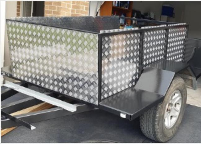
The checker plate is 3mm thick but only weighs 60kg for the sides and lid together; it is a little weird to experience. The aluminium is attached to the metal frame with a combination of Sikaflex automotive adhesive and 5mm stainless steel pop rivets - lots of pop rivets!
