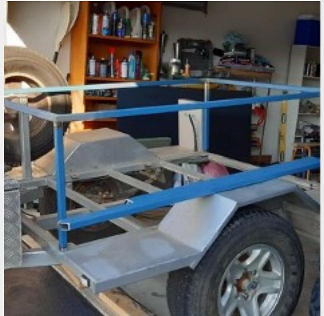
The frame structure is 30mm square tube with a 3mm sidewall. I wanted a trailer with a lid so I could access all the space.
