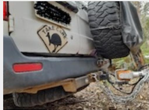
At the very back, I have a spare wheel carrier fitted along with a telescopic light and a wheel bin bag over the spare. I still carry a 2<sup>nd</sup> spare underneath for those longer or sometimes harder trips (yes, I have had to both spares on a rare occasion) and I've got an Anderson plug mounted to the towbar to power and recharge an auxiliary battery in the camper.
