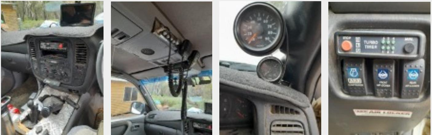
I've also got a couple of gauges installed to monitor the turbo pressure and exhaust gas temperature when driving under load. There are some magic buttons to the side as well to help with traction in slippery conditions and a turbo timer to help cool everything back down at the end of a long drive. I also have an electric brake controller fitted which helps with towing.
