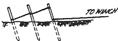
STAKES USED AS GROUND ANCHORS
